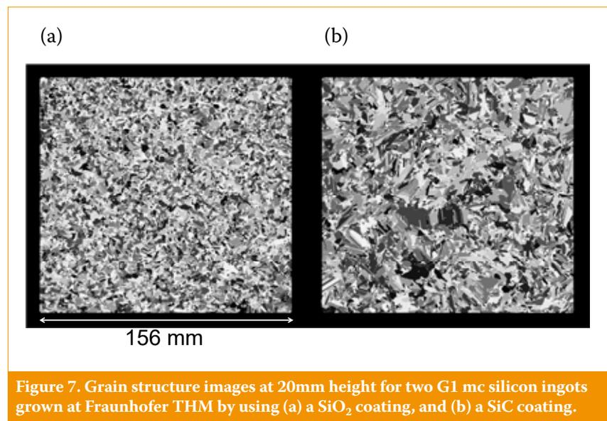
Figure 7. Grain structure images at 20mm height for two G1 mc silicon ingots grown at Fraunhofer THM by using (a) a  $\text{SiO}_2$  coating, and (b) a SiC coating.
