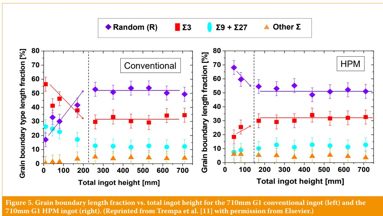
Figure 5. Grain boundary length fraction vs. total ingot height for the 710mm G1 conventional ingot (left) and the 710mm G1 HPM ingot (right). (Reprinted from Trempa et al. [11] with permission from Elsevier.)
