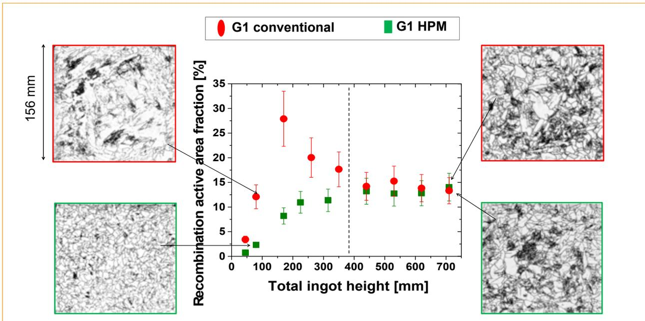
Figure 6. Recombination-active area fraction vs. total ingot height for the 710mm G1 conventional ingot (red circles) and the 710mm G1 HPM ingot (green squares). Photoluminescence (PL) images of both 710mm G1 ingots are shown for total ingot heights of 80mm (left side) and 710mm (right side). (Reprinted from Trempa et al. [11] with permission from Elsevier.)
