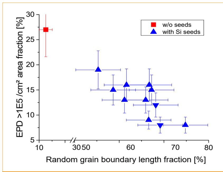
Figure 4. Fraction of areas with an etch pit density (EPD) >1E5/cm² vs. the random grain boundary length fraction at an ingot height of 25mm, for lab-scale HPM material experiments performed without and with silicon seeds. (Data adapted from Reimann et al. [15] with permission from Elsevier.)
