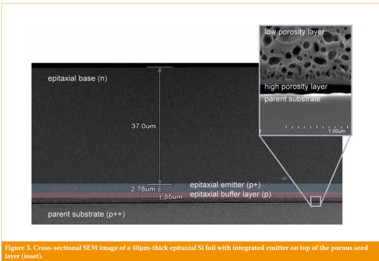
Figure 3. Cross-sectional SEM image of a  $40\mu\text{m}$ -thick epitaxial Si foil with integrated emitter on top of the porous seed layer (inset).
