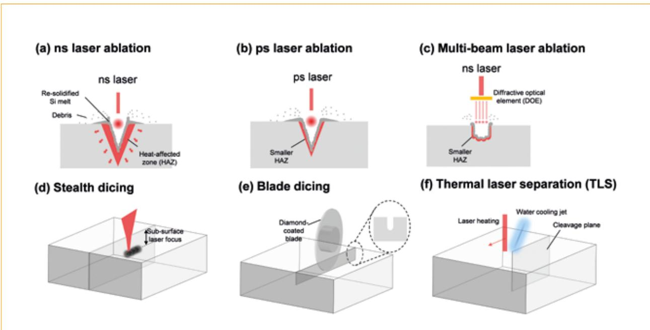
Figure 4. Different delineation methods for defining the area of the epitaxial silicon to be lifted off: (a) nanosecond laser ablation (LA), (b) picosecond LA, (c) multi-beam LA, (d) stealth dicing, (e) blade dicing, and (f) thermal laser separation (TLS).
