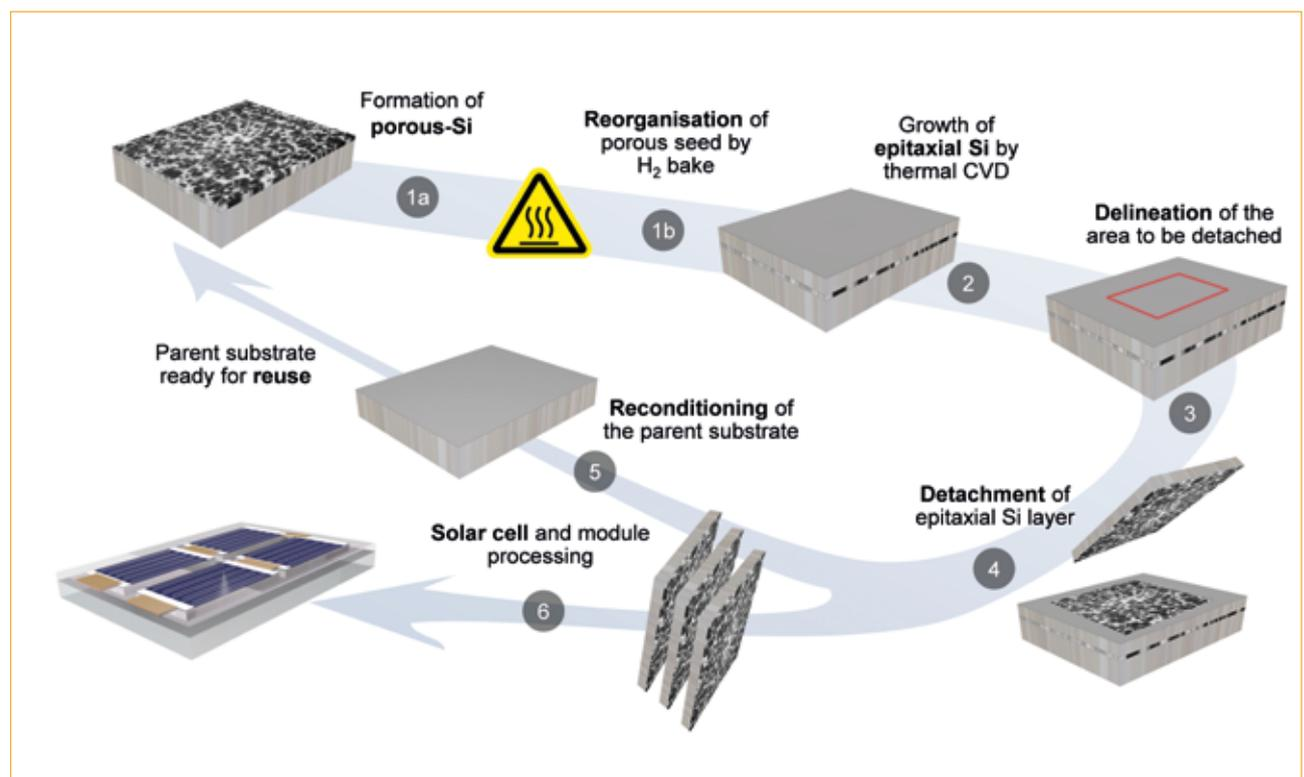
Figure 1. Fabrication of epitaxial Si solar cells and modules from porous-silicon-based epitaxial Si lift-off.
