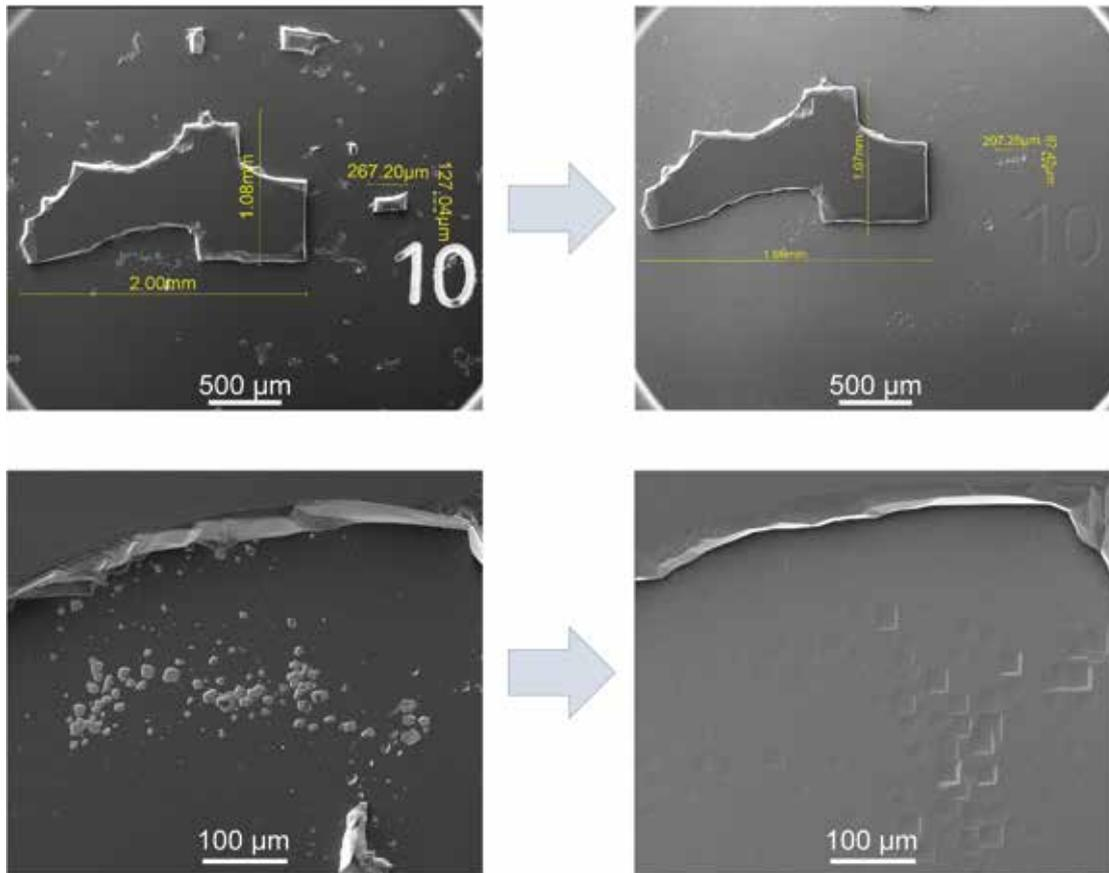
Figure 8. Upon reconditioning by wet chemical etching (here 5μm was removed by TMAH), micrometre-scale defects (such as pillars) are easily dissolved and the surface smoothed out, while larger detachment defects (leading to undetachable epitaxial silicon remnants) remain. Specific markers, such as ‘10’, were used to locate the same region before and after reconditioning.
