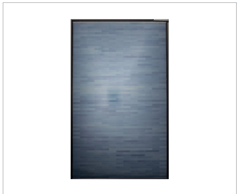
Figure 16. Top view of a bifacial matrix-shingled module (60-cell equivalent, rear side).
