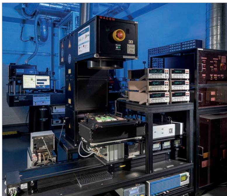
Figure 2. CalTeC's I-V curve measurement facility. A sun simulator provides a class AAA solar spectrum, while an x-z stage allows irradiation of the reference cell, the spectral radiometer or the solar cell under test.
