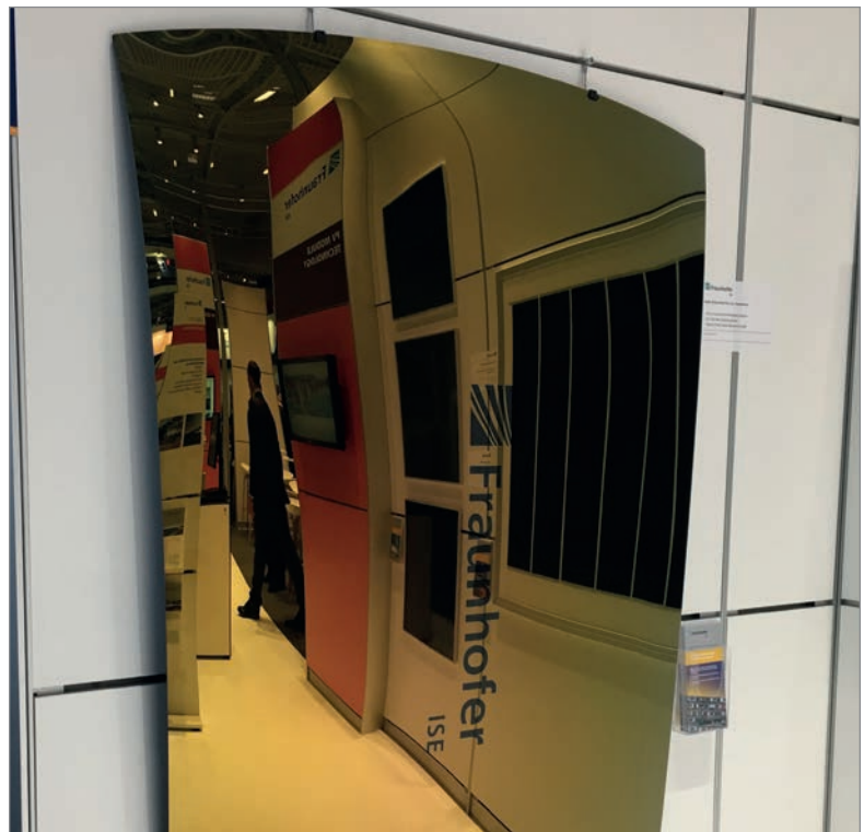
Figure 19. Curved matrix-shingled car roof module presented at Intersolar 2019.
