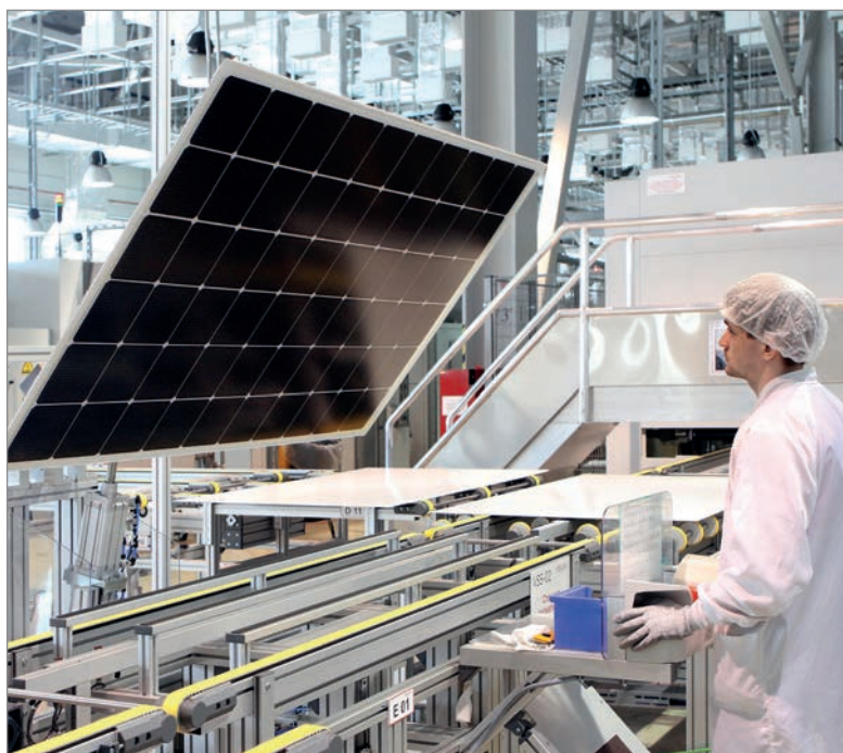
Figure 6. Visual control station on Hevel’s production line.
