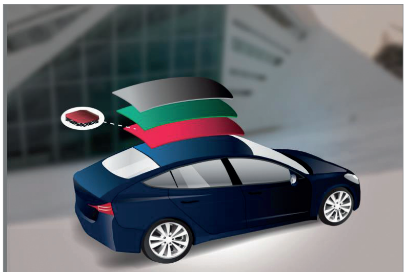
Figure 20. Illustration of an integrated PV-active car roof.
